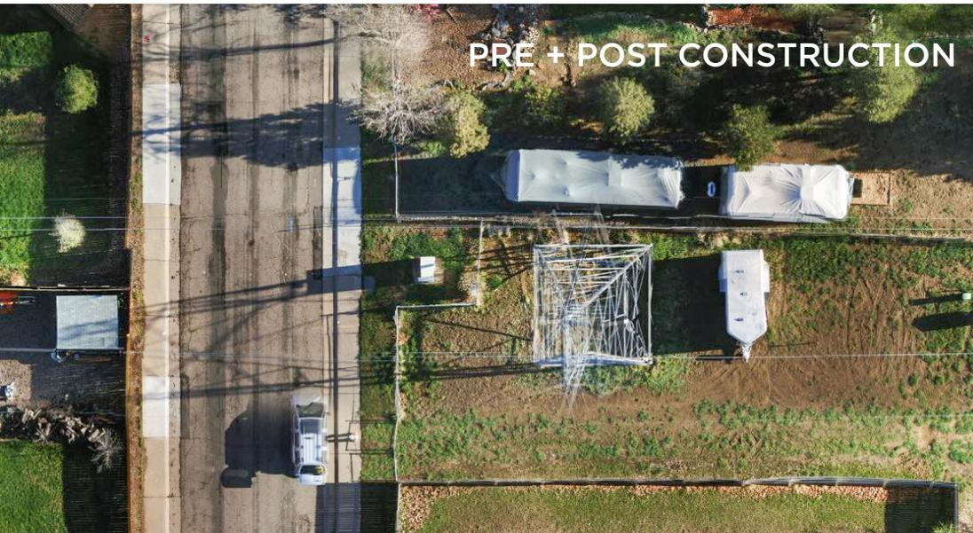
Documenting pre and post-construction conditions avoids liability for pre-existing damage to energized line rights of way, including private and civic property. High resolution UAS imagery can detect even the smallest cracks in access roads.
